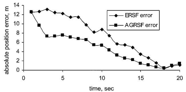
**Fig. 4** Absolute error in position for typical run in BOT problem
