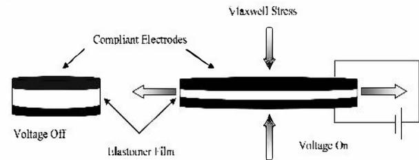
Figure 1 Schematic illustration of dielectric elastomeric actuation
