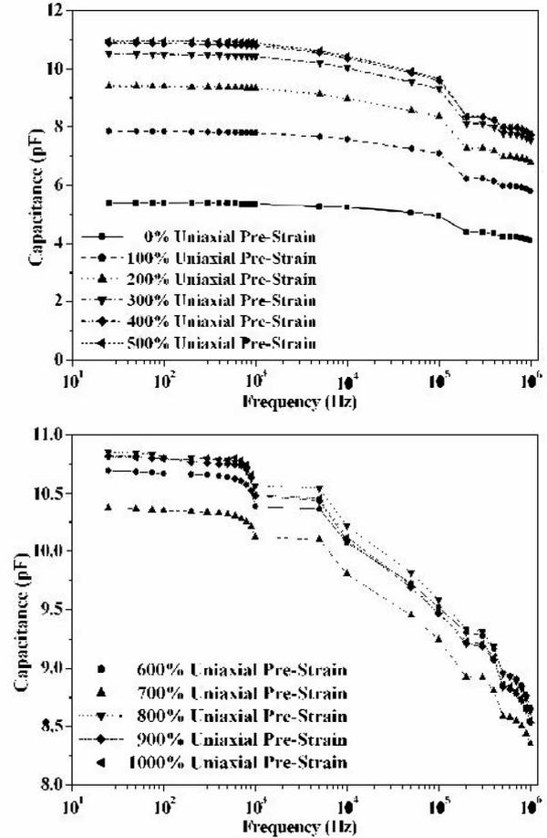
Figure 5 Plot of capacitance as a function of frequency for different uniaxial pre-strain values
