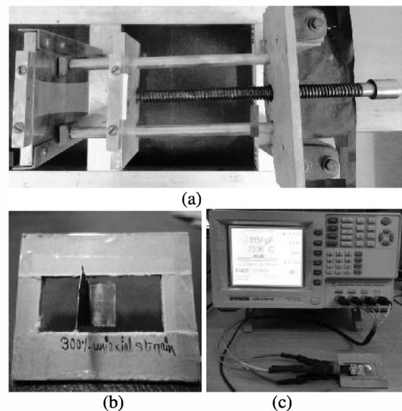
Figure 2(a) Uniaxial stretching device (b) Sample with electrode (c) LCR meter with sample
