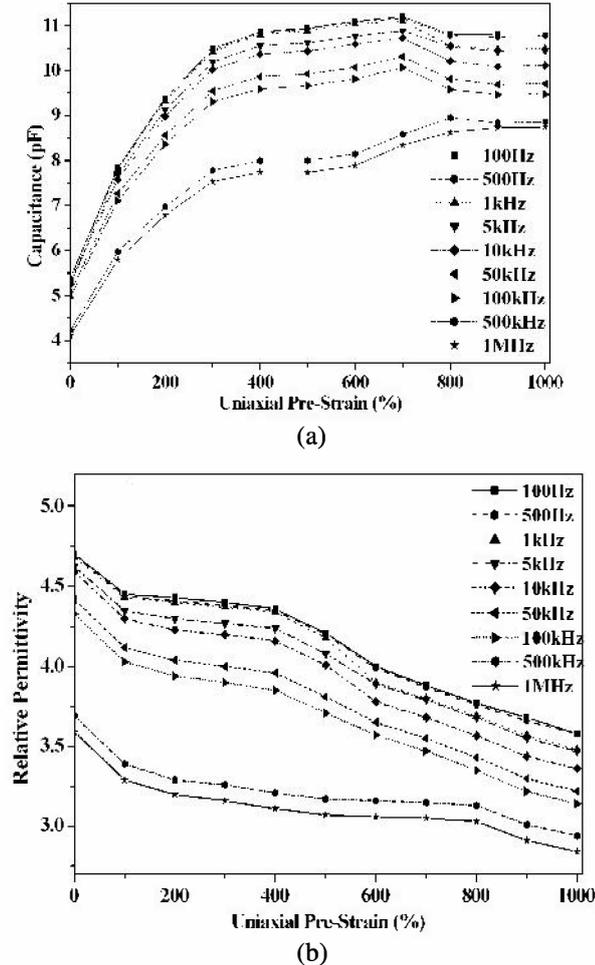
Figure 4 (a) Plot of capacitance versus uniaxial strain at different frequency (b) Plot of permittivity versus uniaxial strain at different frequency
