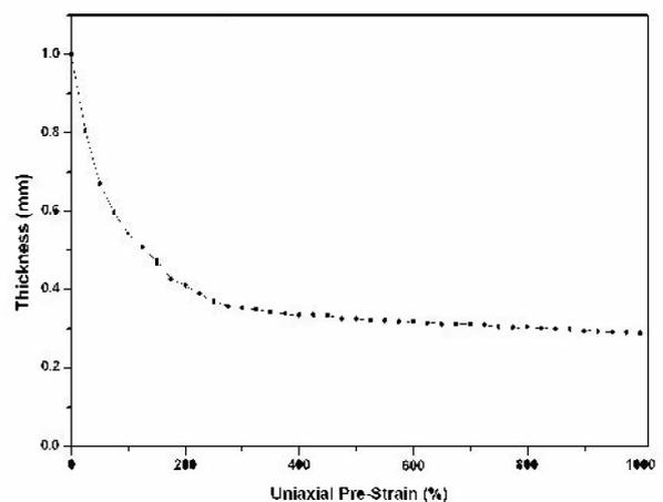
Figure 3 Plot of thickness against the pre-strain
