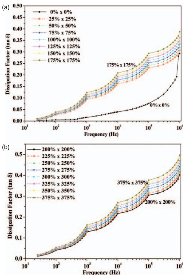
**Figure 3.** Dissipation factor versus frequency for different biaxial pre-strain values using carbon grease electrode.
