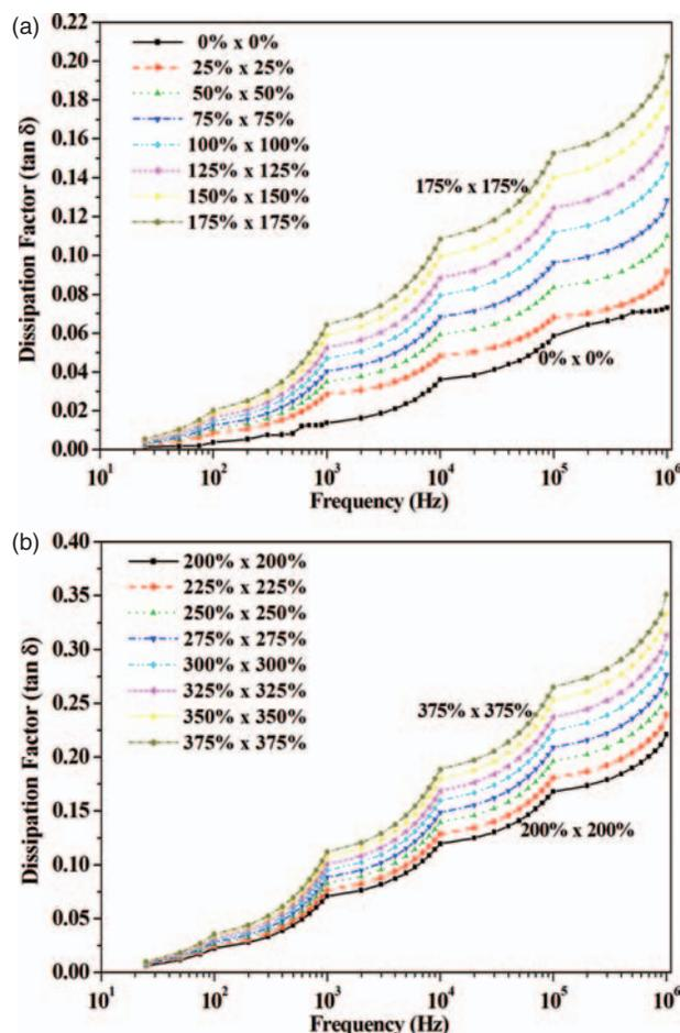
**Figure 4.** Dissipation factor versus frequency for different biaxial pre-strain values using copper tape electrode.
