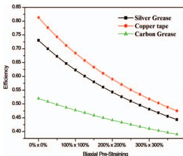
**Figure 8.** Electrical efficiency versus biaxial pre-strain for three different electrode coating at frequency 1 MHz.
