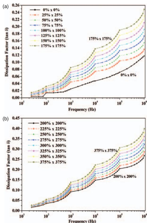
**Figure 5.** Dissipation factor versus frequency for different biaxial pre-strain values using silver grease electrode.
