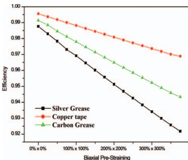
**Figure 7.** Electrical efficiency versus biaxial pre-strain for three different electrode coating at frequency 25 Hz.
