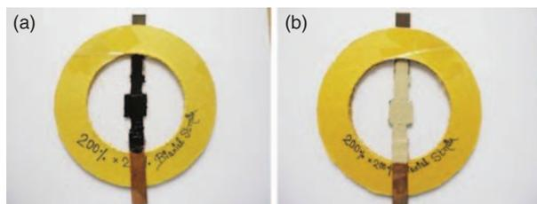
**Figure 1.** 200%  $\times$  200% biaxial pre-stretched samples with (a) carbon grease (b) silver grease electrode.
