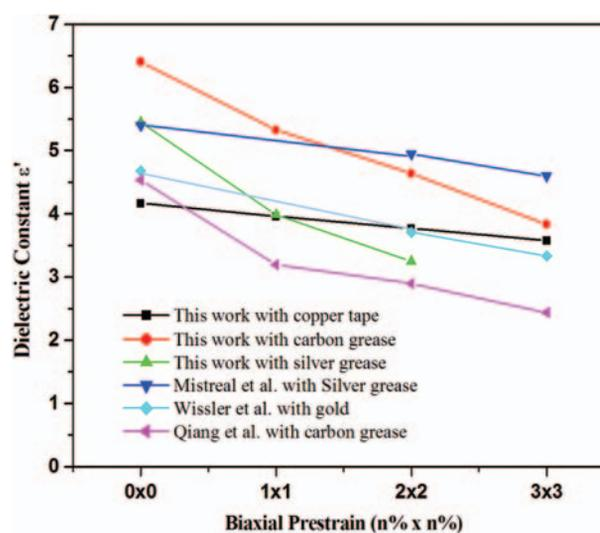
**Figure 6.** Dielectric constant versus biaxial strain at different frequency.
