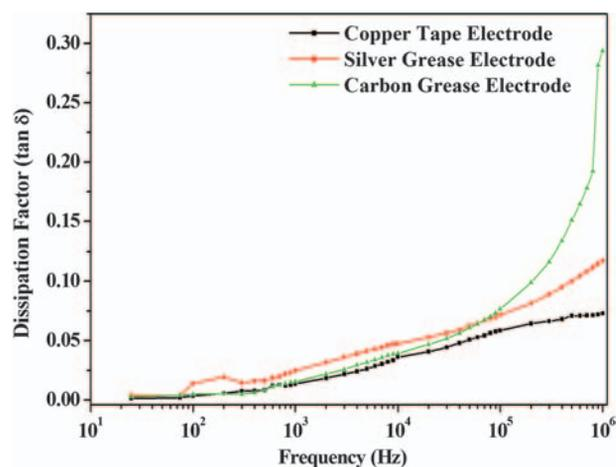
**Figure 2.** Dissipation factor ( $\tan \delta$ ) with frequency for un-stretched sample coated with three different electrodes.
