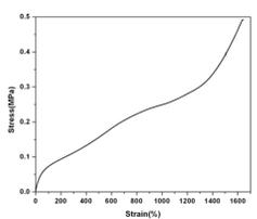
Stress-strain curve for VHB 4910(3M)
