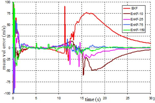
Fig. 6. Mean error of velocity out of 100 MC runs obtained from EKF and EnKF with different ensemble size
