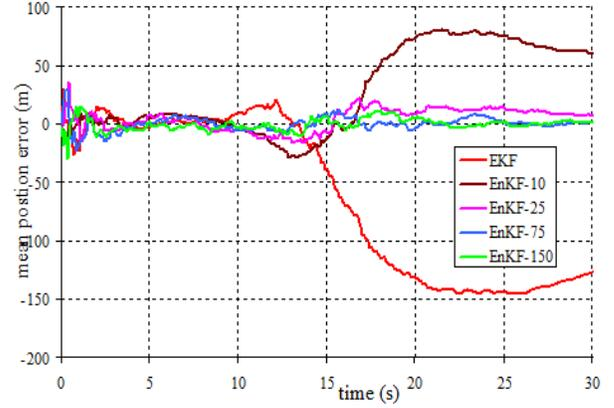
Fig. 5. Mean error of position out of 100 MC runs obtained from EKF and EnKF with different ensemble size
