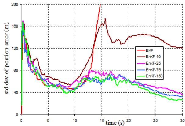
Fig. 8. Std. of position estimation error obtained from 100 MC runs
