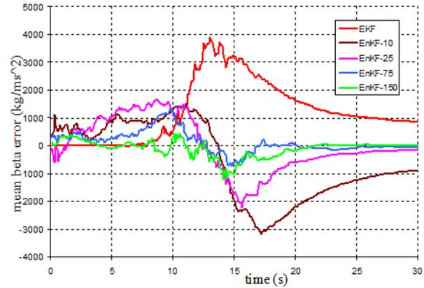
Fig. 7. Mean error of  $\beta$  out of 100 MC runs obtained from EKF and EnKF with different ensemble size
