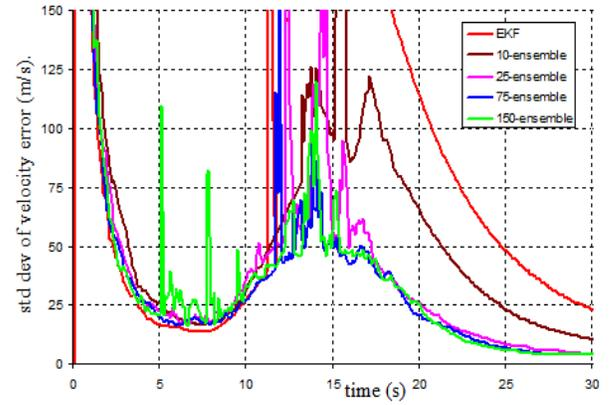
Fig. 9. Std. of velocity estimation error obtained from 100 MC runs
