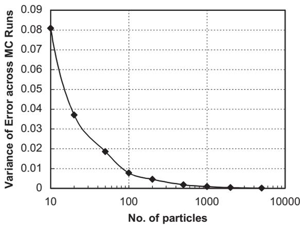
Fig. 1. Convergence of RSPF for 1D nonlinear system and measurements with Gaussian noise.
