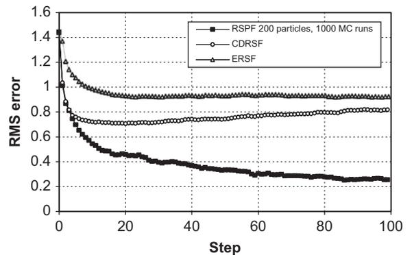
Fig. 4. RMS error settling performance of the ERSF, CDRSF and RSPF over 1000 Monte Carlo runs.
