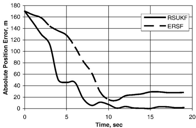
**Figure 4** Absolute value of position error of ERKF and RSUKF in case of large initial position error
