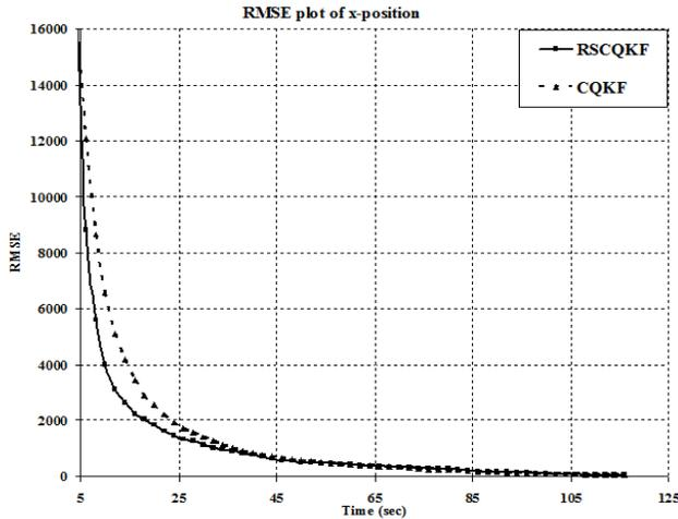
Fig. 4. RMSE plot of RSCQKF (solid line) versus CQKF (dashed line) for x-position of the target
