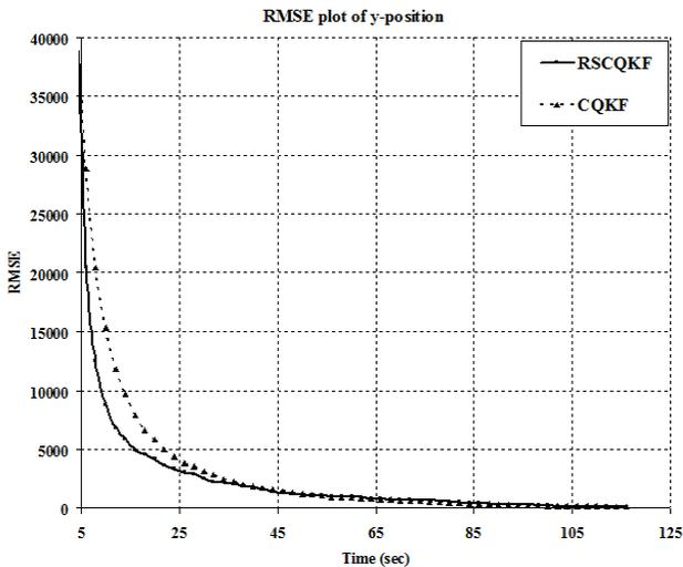
Fig. 5. RMSE plot of RSCQKF (solid line) versus CQKF (dashed line) for y-position of the target
