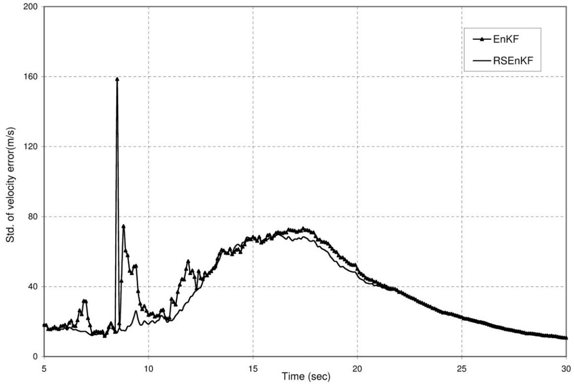
Fig. 8. Std. of velocity estimation error obtained from 50 MC runs.
