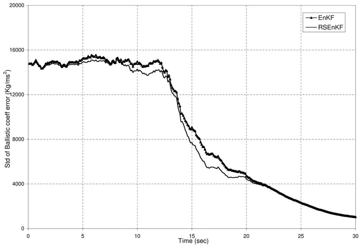
Fig. 9. Std. of ballistic coefficient estimation error obtained from 50 MC runs.
