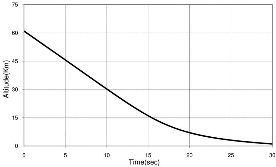
Fig. 4. Typical target trajectory—altitude vs time.
